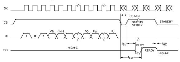
clear cycle of the selected memory location. The clocking of the SK pin is not necessary after the device has entered the self clocking mode. (Note 1.) The ready/ busy status of the CAT93HC46 can be determined by selecting the device and polling the DO pin. Once cleared, the content of a cleared location returns to a logical "1" state.
