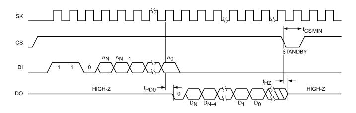
The format for all instructions sent to the device is a logical "1" start bit, a 2-bit (or 4-bit) opcode, 6-bit byte/ word address (an additional bit when organized X8) and for write operations a 16-bit data field (8-bit for X8 organizations).
